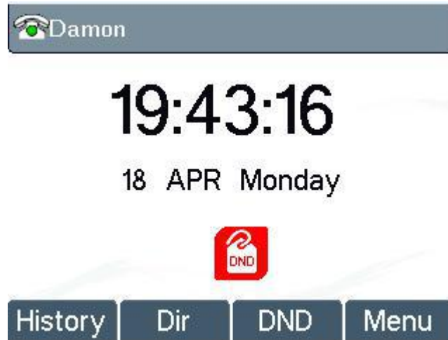
Figure 57 - DND Enabled on All Lines
